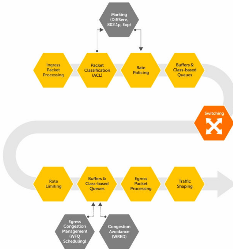
Figure 99. Dell Networking QoS Architecture
